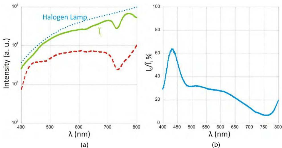
Fig. 6. Spectra of  $\bar{I}_i(\lambda)$  and  $I_o(\lambda)$  (a), and spectral response of the interrogation system (b). In (a), the upper dashed blue line represents the emission spectrum of the halogen lamp WLS. The spectral region of interest for our application is 500-600 nm.
