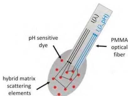
Fig. 1. Drawing of the probe configuration:  $I_i(\lambda)$  is the interrogation light absorbed and scattered by the sensing hybrid matrix;  $I_o(\lambda, \text{pH})$  is the outgoing light containing the information of interest.
