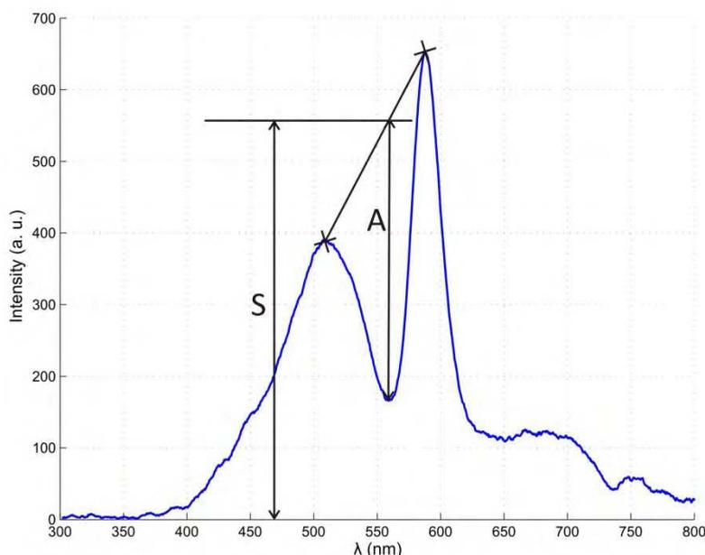
Fig. 11. Graphical definition of the two characteristic parameters. Parameter A is strictly related to the absorption performed by the indicator, whereas S is correlated to the swelling/shrinking processes.
