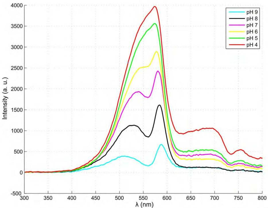
Fig. 10. Spectra of  $\Delta I_0(\lambda)$  acquired at different values of pH. The light absorption of phenol red is well visible at the wavelength of 560 nm. Swelling/shrinking processes induce a change in the amplitude of the whole spectrum.
