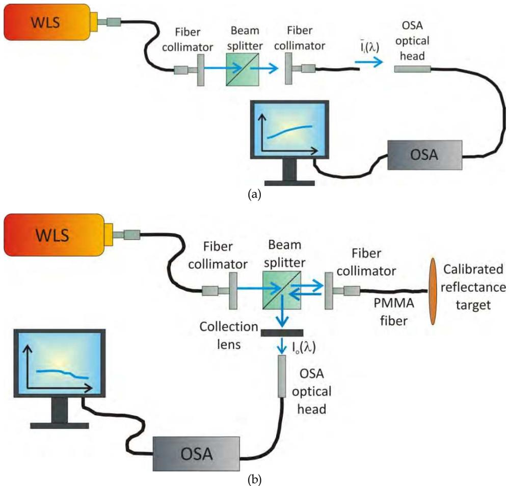
Fig. 4. Experimental setup used to measure the spectral response of the interrogation system. (a) The light spectrum at the output of a 35 cm-long POF without sensing matrix was measured. (b) Afterwards, the spectrometer was reassembled and in front of the POF a calibrated reflectance target acted as a diffuser.
