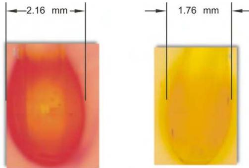
Fig. 9. Two shapes appearance of the probe PEO8000-8:2-PR after 5 min of immersion in basic (left) and acid (right) solution.
