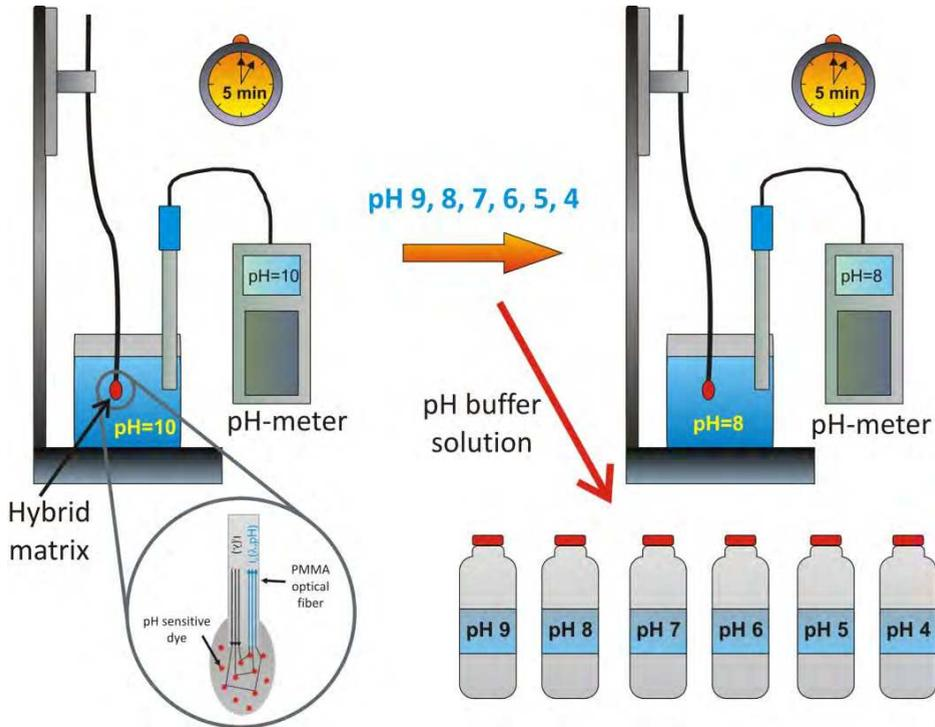
Fig. 5. Schematic representation of the measurement procedure. Firstly, a reference spectrum  $I_0(\lambda, pH_{ref})$  at  $pH_{ref}=10$  was acquired. Then, the pH has been changed from 9 to 4, using standard pH buffers and the response of the disposable sensor has been taken at 5 min after changing the pH level, monitored with the reference pH meter.
