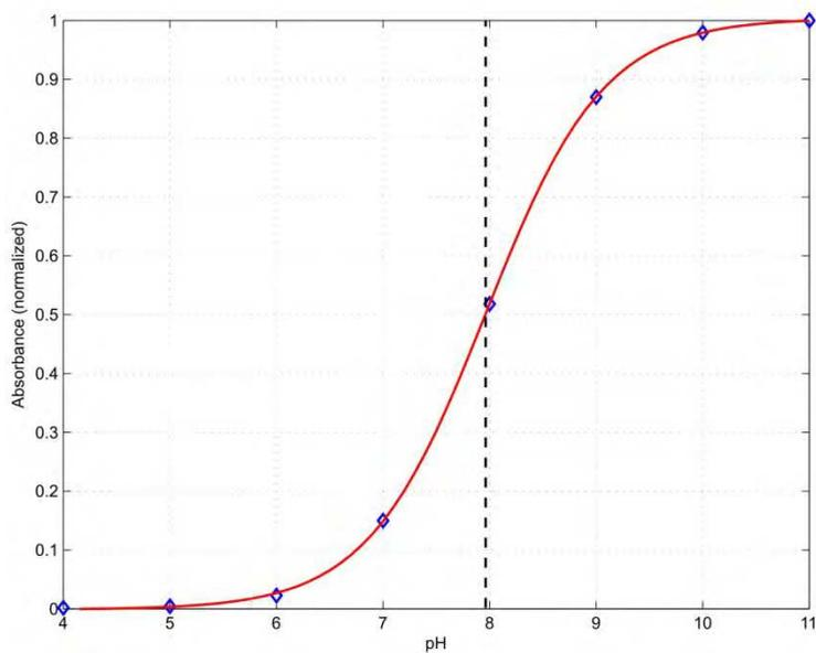
Fig. 8. Absorbance versus pH and Boltzmann interpolation function.
