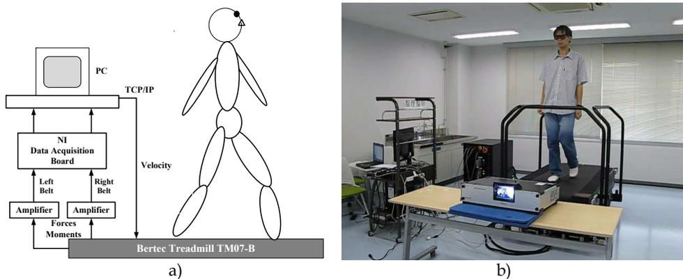
Fig. 10. System construction of human walking servo robot.
