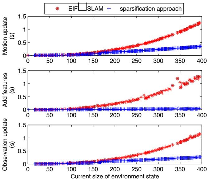
Fig. 4. Efficiency comparison between EIF-SLAM and sparsification SLAM.
