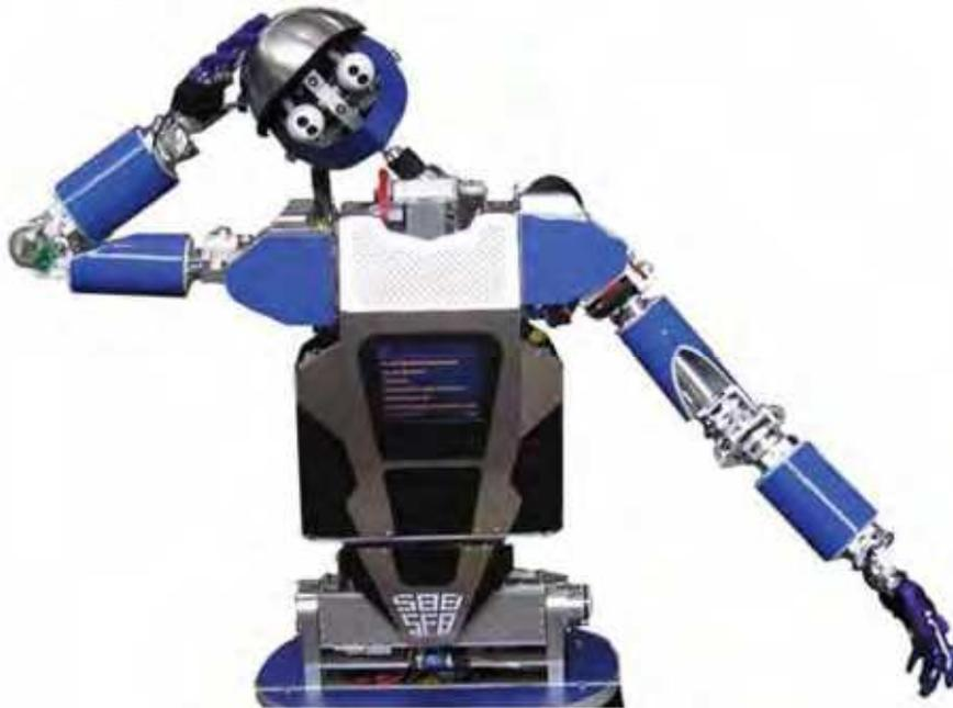
Fig. 6. The upper body of the humanoid robot ARMAR III.
