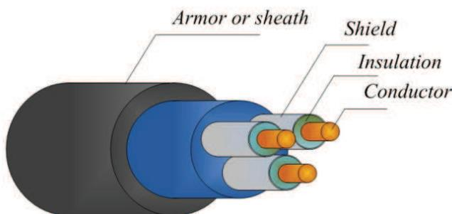
Fig. 1. Generic representation of an electric power cable
