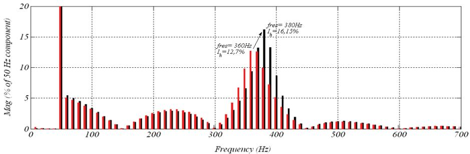
Fig. 17. Harmonic currents at the PCC in function of the location of the harmonic voltage source within the inter turbine grid. For the 30<sup>th</sup> wind turbine (red) and for the 25<sup>th</sup> wind turbine (black)
