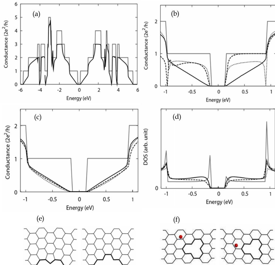
Fig. 8. (a) Conductance of an armchair nanoribbon  $N=8$  with the vacancy type B. (b) Comparison of the conductance of plot (a) with those of the nanoribbon with one and two atom vacancy at the edge (structures of (e)). (c) Comparison of the conductance of plot (a) with those of adatom-vacancy defects of type A-A and B-B (structures of (f)).
