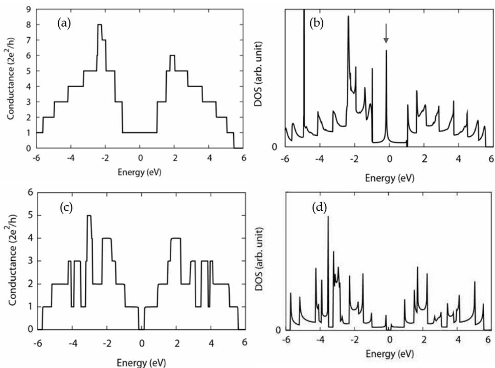
Fig. 4. (a) Conductance and (b) DOS of a zigzag nanoribbon  $N=6$ . (c) Conductance and (d) DOS of an armchair nanoribbon  $N=8$ . The Fermi energy is set to zero. The sharp peak specified by an arrow in (a) refers to edge state of the zigzag nanoribbons.
