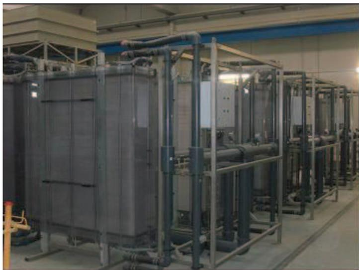
Fig. 4. EDR stacks at the Depurbaix WWTP.
