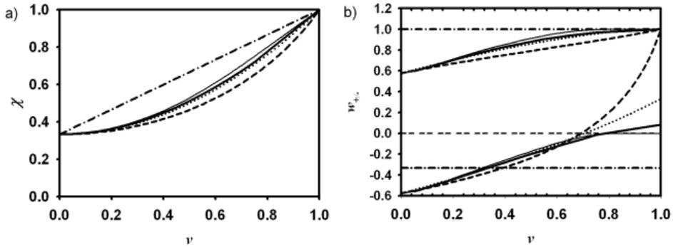
Fig. 4. a) Eddington Factors  $\chi$  versus  $\nu$  and b) characteristic velocities  $w_{\pm}$  for various cases. Minimum entropy production:  $E = E^{(eq)}$  (thick solid curve) and emission limit  $E \ll E^{(eq)}$  (thin solid curve); maximum entropy (dashed); Kershaw (dotted;  $j = 2$  in Eq. (25)), and Auer (dashed-dotted;  $j = 1$  in Eq. (25)).
