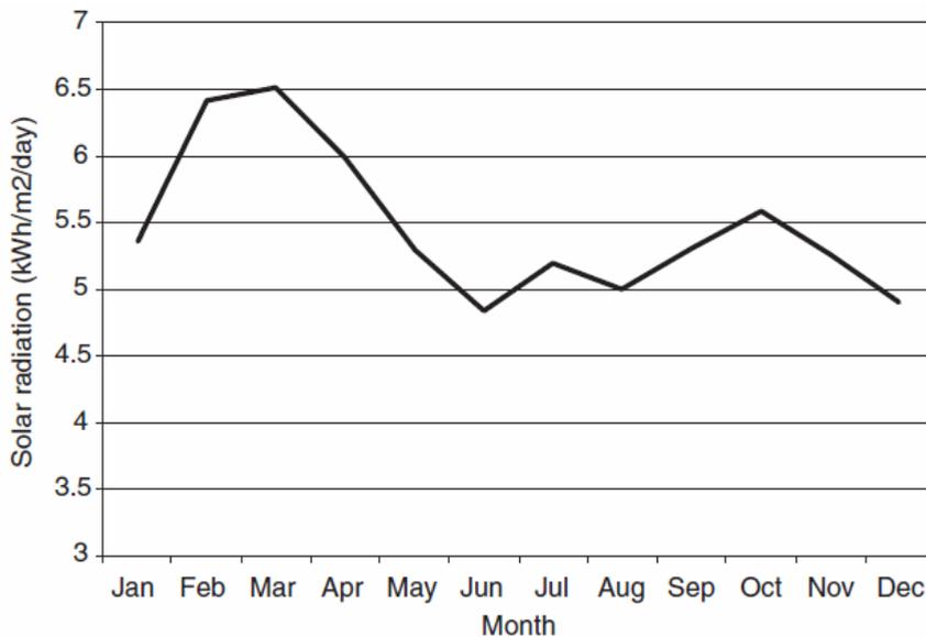
Fig. 7.b Solar radiation levels for locations of pilot installations in Maldives
