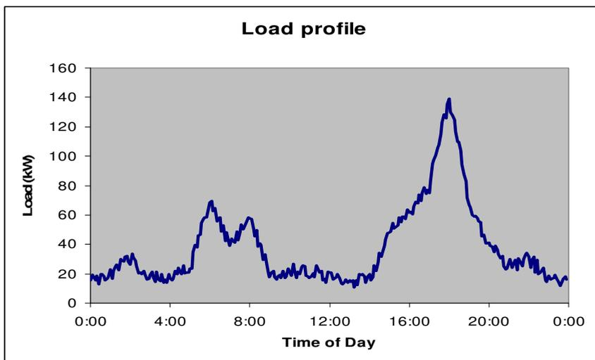
Fig. 1. Typical load profile of a remote community
