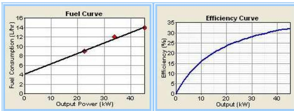
Fig. 2. Typical fuel consumption characteristics of diesel generator
