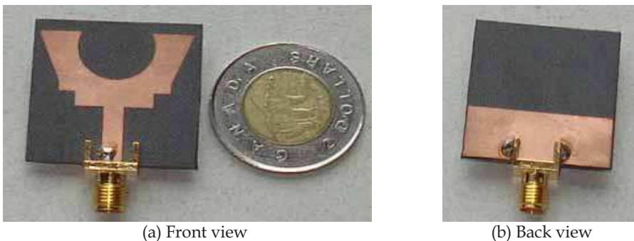
Fig. 5. The prototype of the stepped-trapezoidal patch antenna
