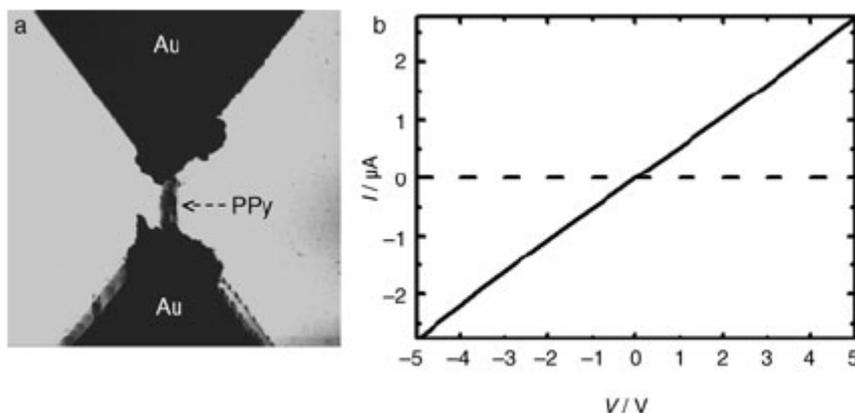
Fig. 1. a) AFM image of a 500-nm-wide polypyrrole wire grown between Au electrodes (image=10-10 mm<sup>2</sup>); b) I-V characteristics of this junction before (b) and after (c) polypyrrole wire growth.
