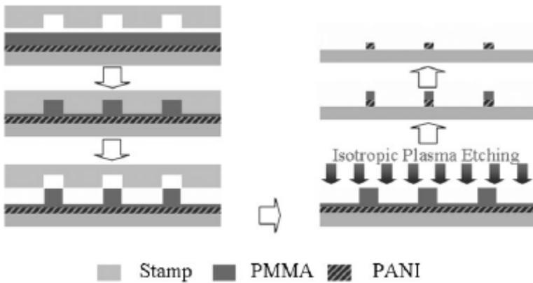
Fig. 7. Schematic illustration of the fabricating process with NIL.
