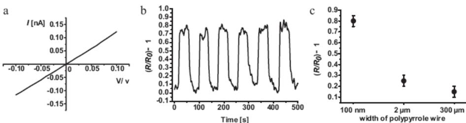
Fig. 5. a)  $I$ - $V$  characteristics of a 100 nm nanodevice consisting exclusively of polypyrrole as shown in Figure 3c. b) Real-time response ( $R/R_0 - 1 =$  sensitivity, see text) of this 100 nm nanowire sensor (Fig. 3c) to a 240 ppm  $\text{NH}_3$  stream (40 s on/40 s off). c) Sensitivity dependence on the width of the wire between the electrodes (at constant thickness).
