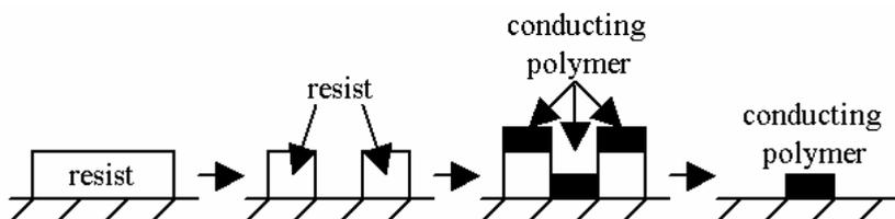
Fig. 2. Schematic representation of the fabrication process.
