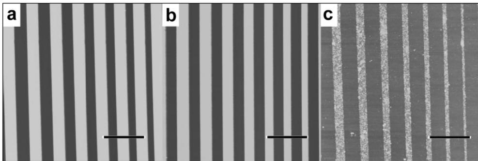
Fig. 8. AFM images of (a) the silicon stamp, (b) an imprinted PMMA structure using the stamp shown in (a), and (c) fabricated PANI structures with NIL (Scale bar=7.5μm).
