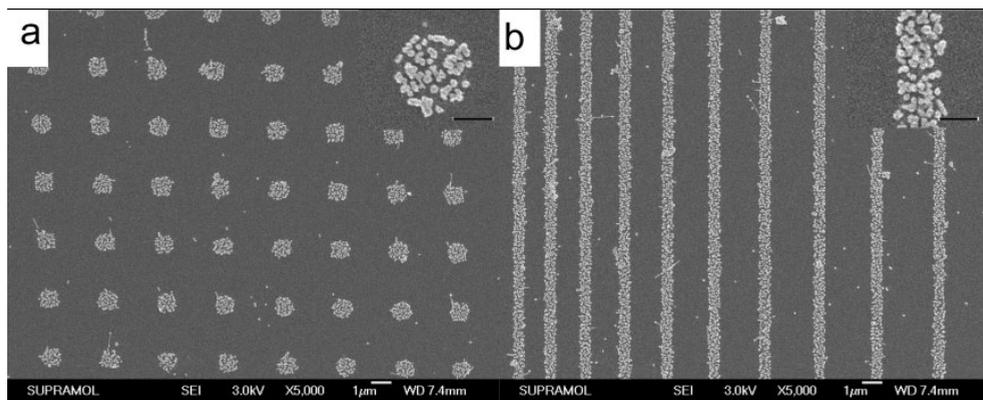
Fig. 10. SEM images of SNPs adsorbed onto the PANI dots (a) and lines (b). Scale bar=1 mm. Scale bar of the insets=500 nm.
