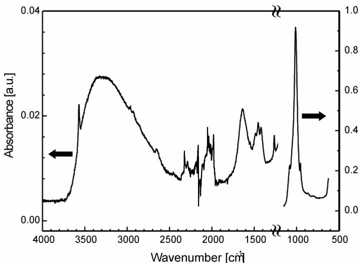
Fig. 9. FTIR spectrum of pure HAp nanorods.
