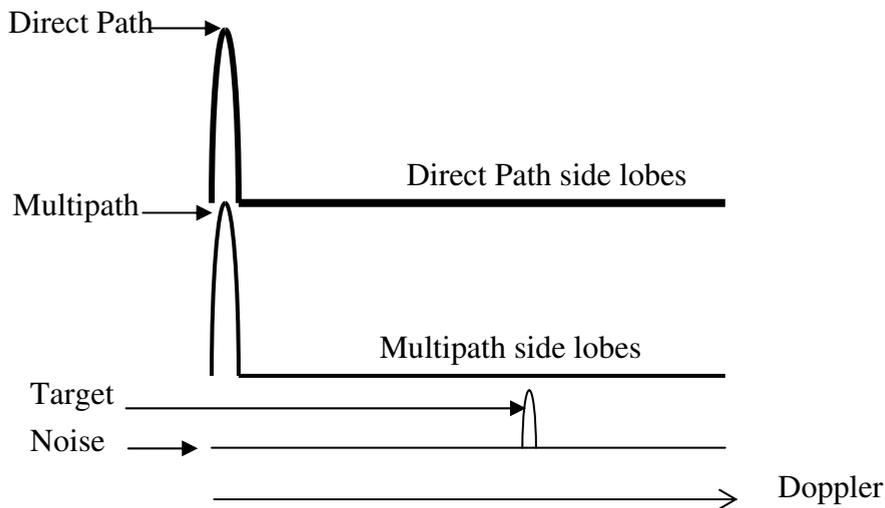
Fig. 3. Schematic radar equation (target hidden by side-lobes).
