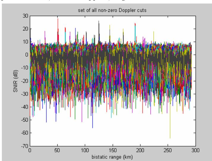
Fig. 10. Non-zero-Doppler cuts (of the range-Doppler correlation) after adaptive filtering
