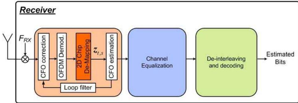
Fig. 9. Fine CFO estimation scheme before despreading function
