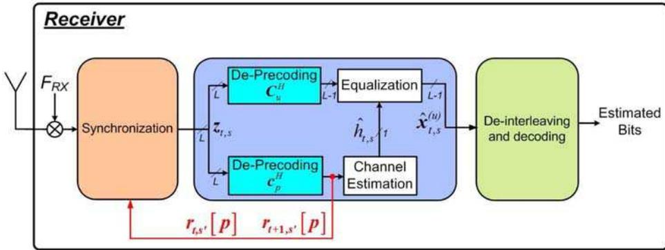
Fig. 11. Joint residual CFO and SFO estimation scheme after the deprecoding function as the function describing the total phase rotation and  $\psi_{t,s'} [q, n']$  as the function describing the amplitude attenuation caused by CFO and SFO on the interested subcarrier.
