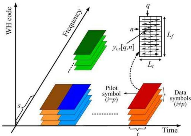
Fig. 3. 2D Spreading Scheme
