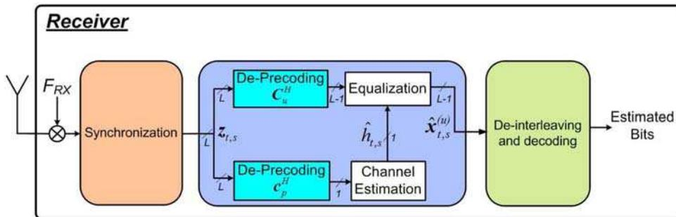
Fig. 4. Channel estimation scheme based on spread pilot
