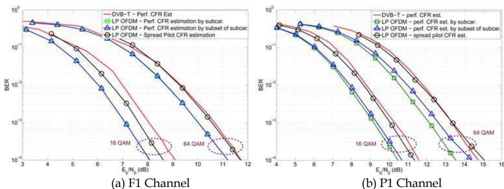
Fig. 7. Performance comparison between the DVB-T system with perfect CFR estimation and the proposed 2D LP OFDM under time-invariant channel models -  $R_c = \frac{1}{2}$  -  $L_f = 4$  and  $L_t = 16$  -  $P_p = 7$
