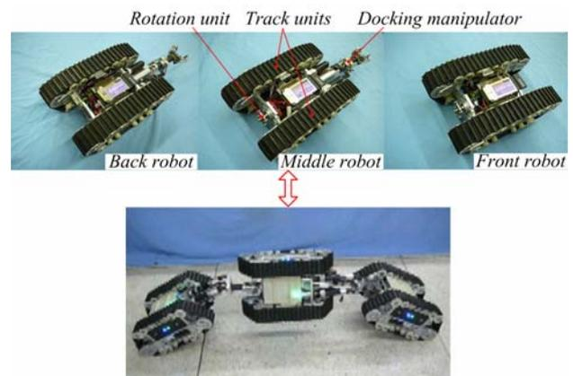
Fig. 1. Three robots in the JL-2 system
