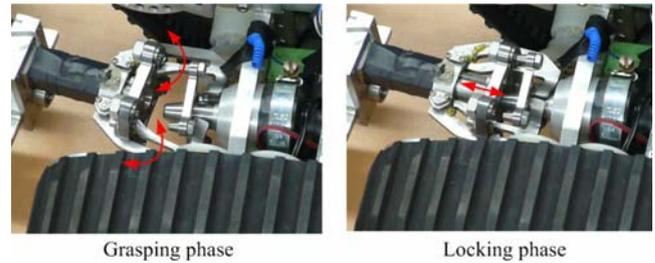
Fig. 5. Two phases in docking procedure
