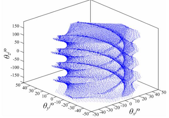
Fig. 7. Available kinematics workspace of the spherical joint
