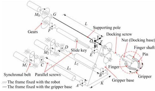
Fig. 2. Kinematic diagram of the docking manipulator
