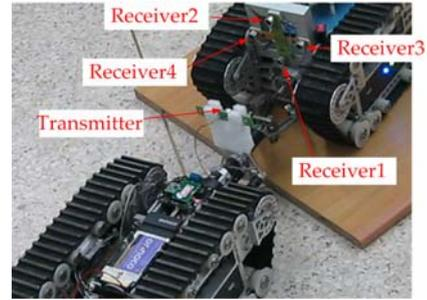
Fig. 10. Sonar sensors for automatic docking
