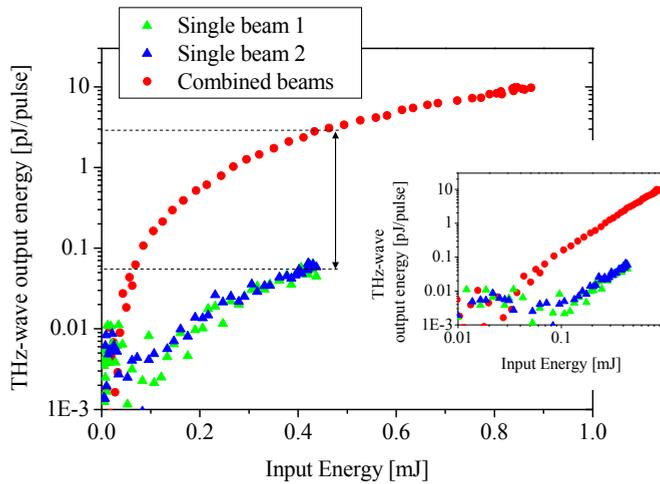
Fig. 14. Input-output property of THz-wave for pumping energy at 1.0 THz generation with  $\alpha=2.49$  degrees. Circles and triangles denotes THz-wave output signal with combined beams and with single beam. Inset shows double logarithmic plot of input-output properties.
