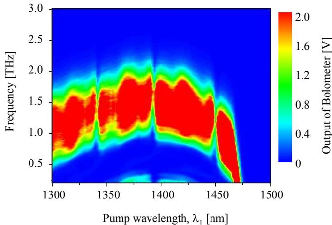
Fig. 4. THz-wave output mapping for various pumping wavelengths and corresponding THz-wave frequencies. The X-axis and Y-axis denote pumping wavelength  $\lambda_1$  and THz-wave frequency, respectively. The magnitude of the map values indicates the output voltage of the detector.
