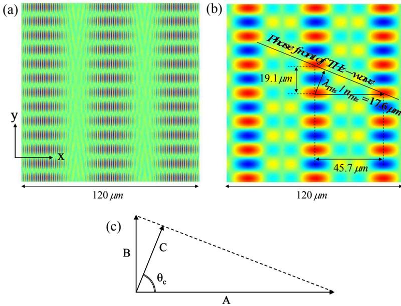
Fig. 11. Normalized electric field distribution of (a) combined dual wavelength pump beams with finite angle, and (b) exited second order nonlinear polarization of difference frequency. Here,  $\lambda_1=1300$  nm,  $\lambda_2=1317$  nm and 3 THz of difference frequency with 3.7 degrees of beam angle. (c) Geometric relation of A: excited nonlinear polarization for x-direction, B: interference period of pump beams for y-direction and C: THz-wavelength in the crystal.
