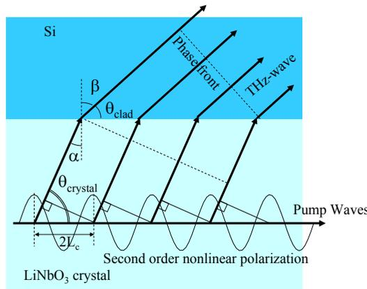
Fig. 1. Schematic of Cherenkov phase-matched monochromatic THz-wave generation.
