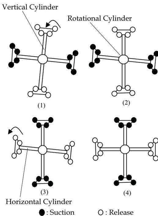
Fig. 5. Rotation of the robot
