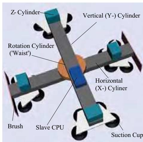
Fig. 2. Main structure of the climbing robot
