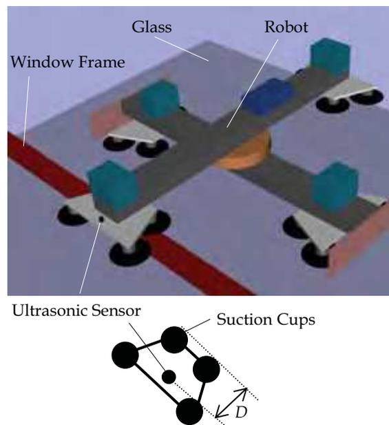
Fig. 7. Ultrasonic sensors installed on the robot
