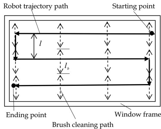
Fig. 4. Robot motion path on the glass
