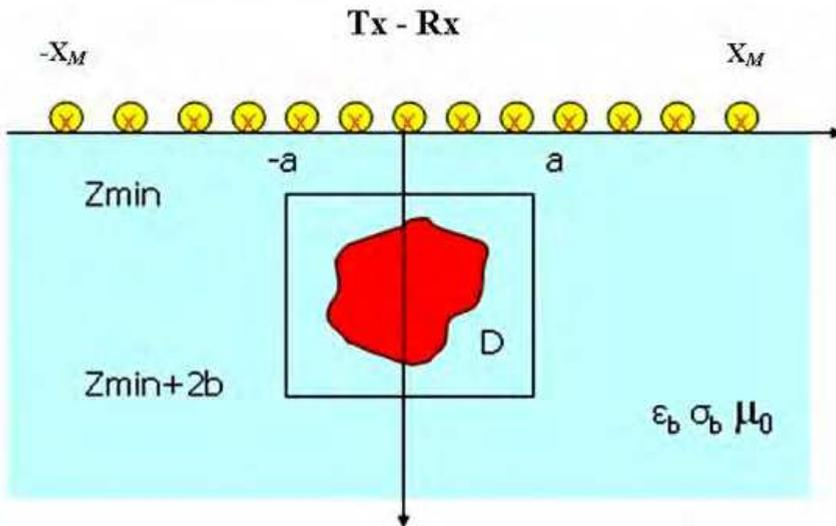
Fig. 6. Geometry of the subsurface prospecting problem
