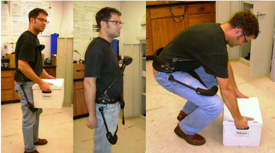
Fig. 9. BNDR lift assist system.
