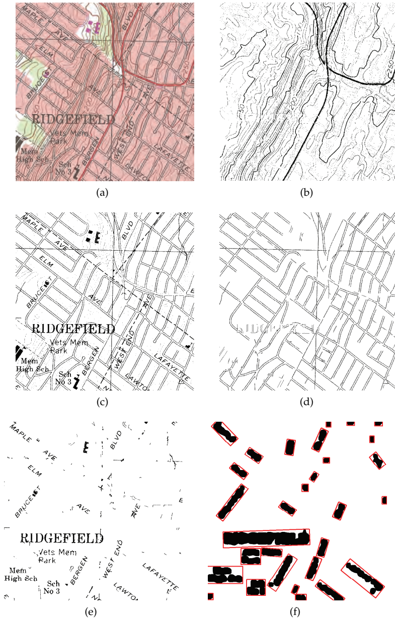
Fig. 1. Performance evaluation of the text and graphics separation modules; (a) Original map image, (b) Extracted Contour Lines, (c) Foreground image, (d) Extracted linear features , (e) Text image, (f) Grouped characters and their respective minimum area enclosing rectangles
