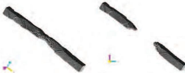
Fig. 4. Tensile Deformation and Failure of 5X5X60 Nickel Nanowire; Strain Rate =  $1.67 \times 10^7$  ( $s^{-1}$ )
