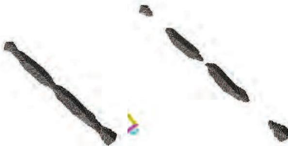
Fig. 5. Tensile deformation and failure of 5×5×60 Nickel nanowires; strain rate= $1.67 \times 10^{10}$  ( $s^{-1}$ )
